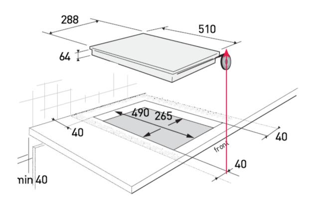
Glue the foam seal underneath your appliance by following the outline of the work top upon which your appliance will rest to ensure a snug fit.
