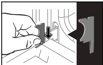
Remove the first clipped window: use a tool (screwdriver) in the slots (**A**) to unclip the window and then remove it.
