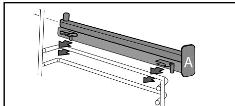
NOTE: the telescopic sliding part of the rail must unfold towards the front of the oven, with the buffer **A** opposite you.
