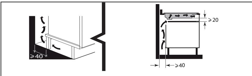
or above a built-in oven, comply with the dimensions provided on the illustrations to ensure a sufficient air outlet at the front.
