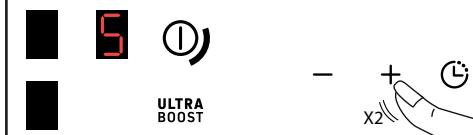
With a power level > 5, a quick double press on the + button allows you to switch directly to power level 9.
