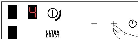
With a power < 5, a quick double press on the + button allows direct access to power 5.
